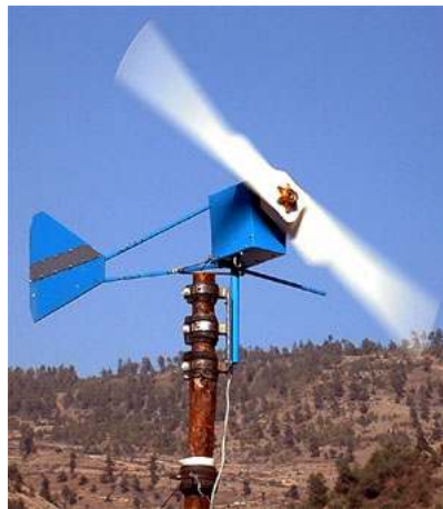
Picture 50: Power generation of maximum 180 watt can be achieved.
