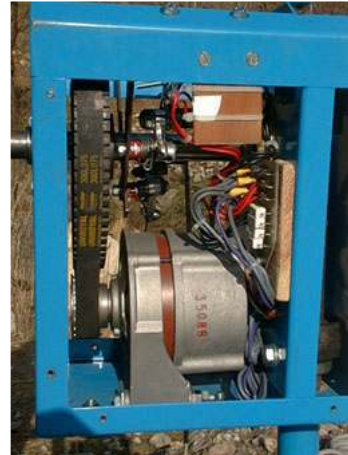
Picture 48: Bosch K1 14 volt 35 amps car alternator, 1:4 wheels with belt set system, capacitors, electronic circuit plate, brakes
