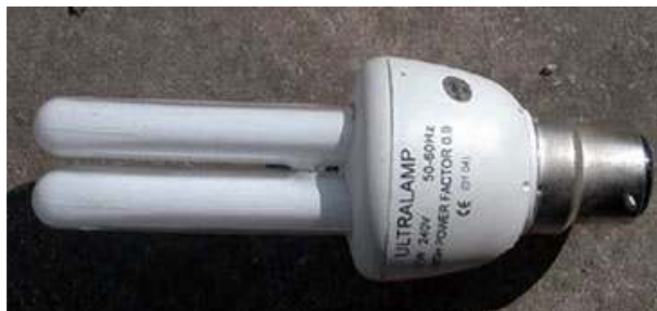
Picture 7: High quality CFL Lamp 11 watt (from Ultralamp), with a high Power Factor (PF) of > 0.9 , and with a life expectancy of 8,000 – 12,000 hours. Its light output can be compared with a 55 watt incandescent bulb.
