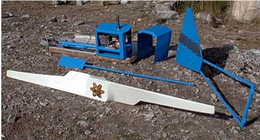
Picture 47: Self made 2 bladed wooden wind turbine, wooden tail with metal frame, and a Bosch car alternator as power generator. The wooden blades are hand carved aerofoil shaped blades with a blade diameter of 205 cm. From ~ 300 Rpm onwards the wind generator provides 12 volts to charge the battery bank.
