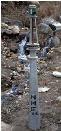
Picture 11: Pico hydro power plant generating 165 watt
