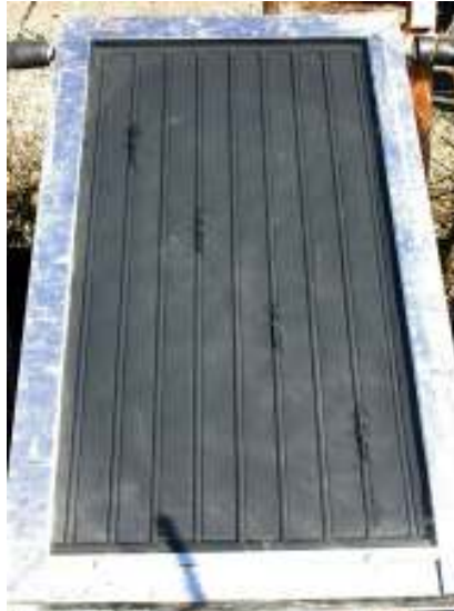
Figure 2-10 Nine ½” GI-pipe raisers with aluminum fins are used as absorber, rather than copper, for sustainability reasons, as copper can not yet properly be welded in Nepal. Four thermocouples at different heights measure the temperature profile on the absorber. The top and sides are overlapped with galvanised sheets while at the bottom the rain can run off freely.
