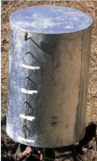
Figure 2-9 The 300 liter, stainless steel hot water storage tank is insulated with 100mm polyurethane foam. The air ventilation valve exits at the top on the side, in order to minimise heat losses. Four thermocouples at different heights in the hot water tank measure the attained stratification.
