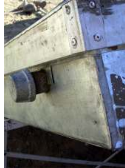
Figure 2-11 A 50mm Styrofoam insulated aluminum lid covers the absorber all around tide, including 50mm overlapping, in order to minimise the absorber heat losses during the freezing nights. The lid’s corners are reinforced to increase its stiffness. The lid acts during the day as a reflector with its high gloss, stainless steel sheet on the inside.
