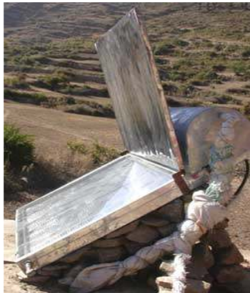
Figure 2-4 The storage tank is integrated to limit pipe heat losses. The insulated, reflecting aluminum lid acts as a night time cover and day time reflector.
