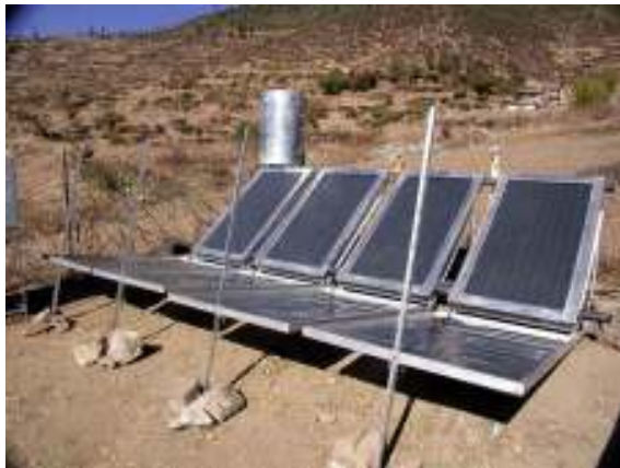
Figure 2-7 The 2 nd Generation Thermo-Siphon HASWH, with opened, adjustable cover lid reflectors. A 40° south angle pyranometer, records the received solar irradiation on the absorber. The absorbers and insulated pipes can be shut off from the storage tank and emptied through hand valves as part of the freezing protection.
