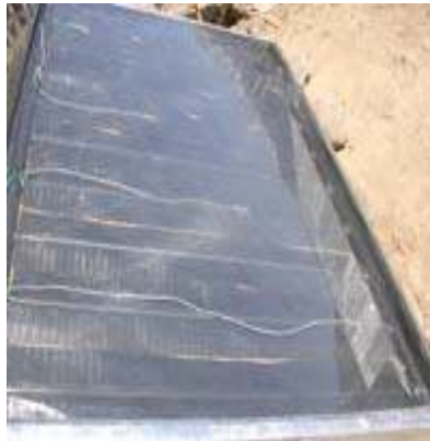
Figure 2-5 Selective coating, copper fin absorber with 4 thermocouples at different heights to record the temperature profile. The normal window glass cover limits the incoming solar radiation to 80%-82%.
