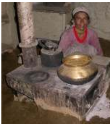
Picture 4: The high altitude smokeless metal stove allows to cook the traditional “dhal bhat” all at one time, saving up to 50% fire wood. It cooks easily for up to 12 people.
