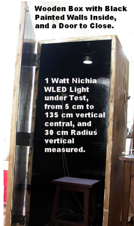
Figure 6-6: Light Box The 160 cm high wooden box with black walls inside.
