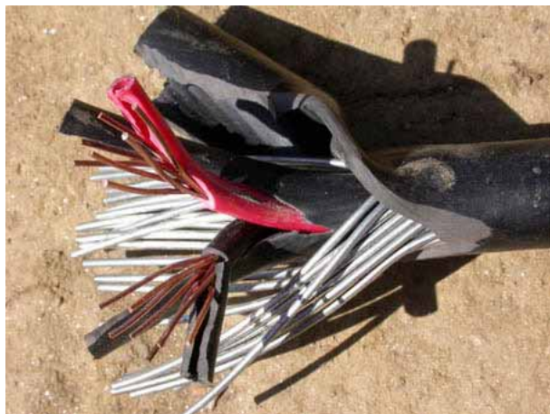
Figure 12-11: Armored Cable 4mm 2 4mm 2 , 2 strings @ 7 copper lids armored cable, able to carry 41 Amp and 1,100 Volt, at up to 70° C conducting temperature. .
