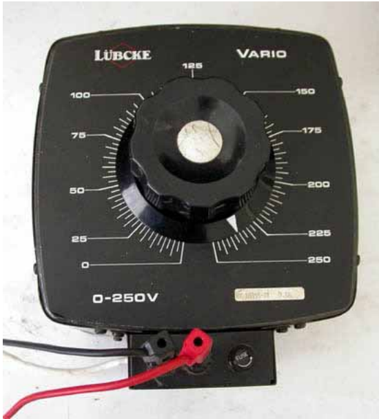
Figure 6-5: Variable Voltage Transformer With this variable voltage transformer for the 25 W, 40 W, 60 W and 100 W incandescent bulbs, as well as for the 7 W, 11 W, and 15 W CFL bulbs were kept constant to provide equal comparable test conditions. The 230 VAC were periodically measured with a multimeter to make assure to have equal conditions for each light bulb.
