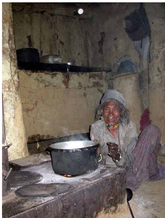
Figure 6-10: Home with Smokeless Metal Stove A home with 3 WLED Lights and a smokeless metal stove for cooking (making a whole meal at the same time through its three burners), providing hot water, and heating at the same time. Thus NO smoke inside the home, NO danger for children, better hygiene (through the hot water) and half the amount of daily fire wood consumption, are the results.
