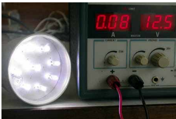
Figure 6-3: WLED Measurement 1 The 9 diodes Nichia WLED light consumes in fact 3 \times 3.6 = 10.8 VDC, @ 70 mA. 12.5 VDC @ 80 mA are constantly provided, in order to be slightly higher than what the WLED light needs. Internal the WLED cuts down the DC voltage to 10.8 VDC. That means that this WLED light consumes 864 mW under the test conditions.
