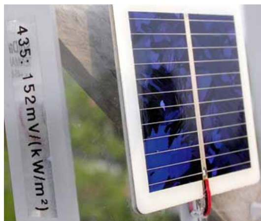
Figure 7-8: 80SPC SolData Pyranometer One of the three SolData 80SPC silicon photovoltaic pyranometer.
