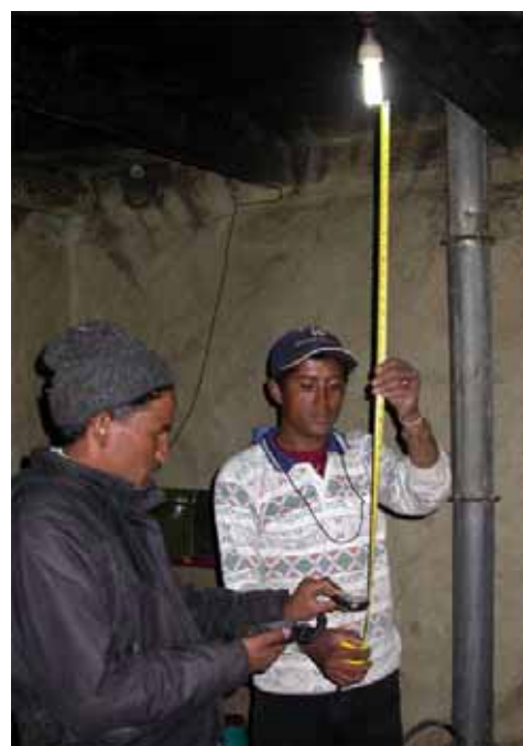
Figure 5-2: CFL Light Output Measurement
