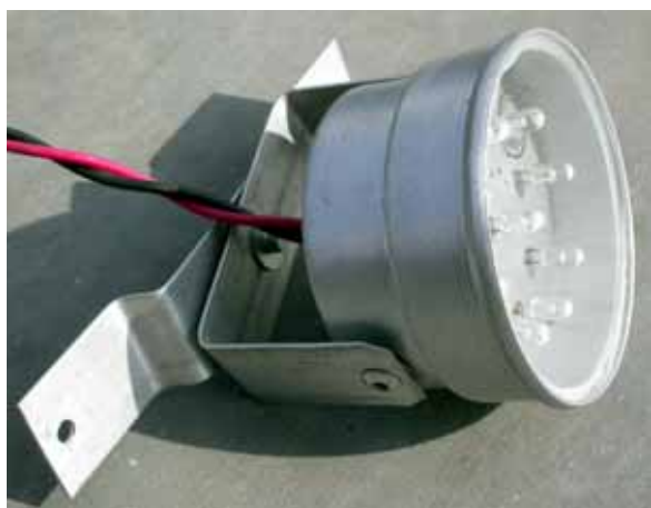
Figure 12-12: Nichia WLED Light The WLED lights are manufactured by PPN in Nepal. One WLED light has 9 individual Nichia NSPW510BS WLEDs with an angle of 50°. The light can be moved around two axis to adjust the light beam inside the home.
