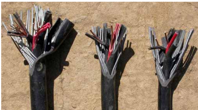
Figure 12-10: Armored Cable 4mm 2 , 2.5mm 2 , 1.5mm 2 The three different sized armored (with galvanised armored steel wire) copper underground cables used in the Chauganphaya Solar PV System transmission lines. The 2 copper strings are with PVC insulated. Inside and outside is a PVC covering layer, providing additional protection. The cables are manufactured in Nepal.
