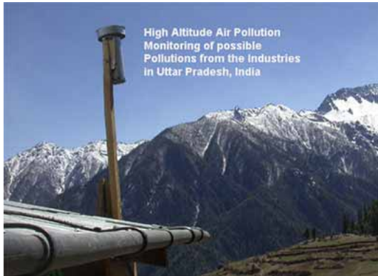
Figure 7-25: Air Pollution Sampler In collaboration with the University of Manitoba in Canada, a newly started air pollution sampling project has started with 2 samplers, to monitor the possible air pollutions in high altitude Himalayan regions in one year time periods. Possible expected pollutions come from the uncontrolled pollution generation of India's massive growing heavy industries in the northern territories of India. The states most probably affecting Nepal's Himalayan regions are, Bihar and Uttar Pradesh (India's biggest populated state), both along side Nepal's southern boarder.
