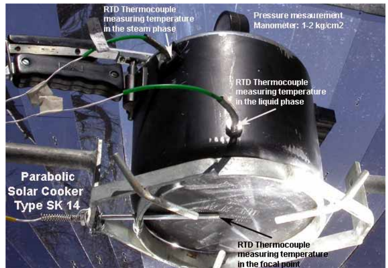
Figure 7-24: Parabolic Solar Cooker SK 14 SK 14 Solar Cooker with 4 monitoring parameters, all with RTD type thermocouples (made in India). One RTD measures the temperature of the parabolic solar cooker's focal point. One RTD measures the lower, liquid part of the food cooked inside the pressure cooker. One RTD measures the upper, steam part of the food being cooked. A 1 – 2 bar absolute pressure manometer provides an instant reading of the pressure cooker inside pressure.
