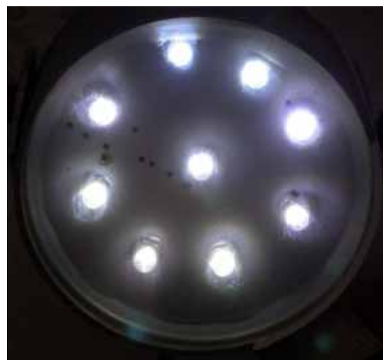
Figure 12-26: WLED Light On Each of the 9 WLEDs consumes 20-25mA @ 3.6VDC. That amounts to ~800mW for a 9 WLED Nichia light as installed in the Chauganphaya village homes. Allowing some power transmission losses means that 1 Watt power consumption with about 23 lumens illuminance can be accounted for.
