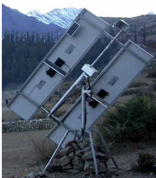
Figure 12-20: 2-Axis Self-Tracking Frame 2 2-axis self-tracking frame right after sunset. The tracker has a minimum azimuth angle of -170^{\circ} (fully East), and a maximum azimuth angle of 10^{\circ} (fully West as in the Figure). Thus the tracker tracks the sun over an angle of 160^{\circ} during the course of one full sunny day. During the spring season (March – May) every year strong winds occur due to the intensive thermal movements of the upraising air from the ground. In order to hold the frame and solar PV modules secure, the tracking frame is constructed at its base in such a way that it can be filled with a pile of stones, once it is installed.
