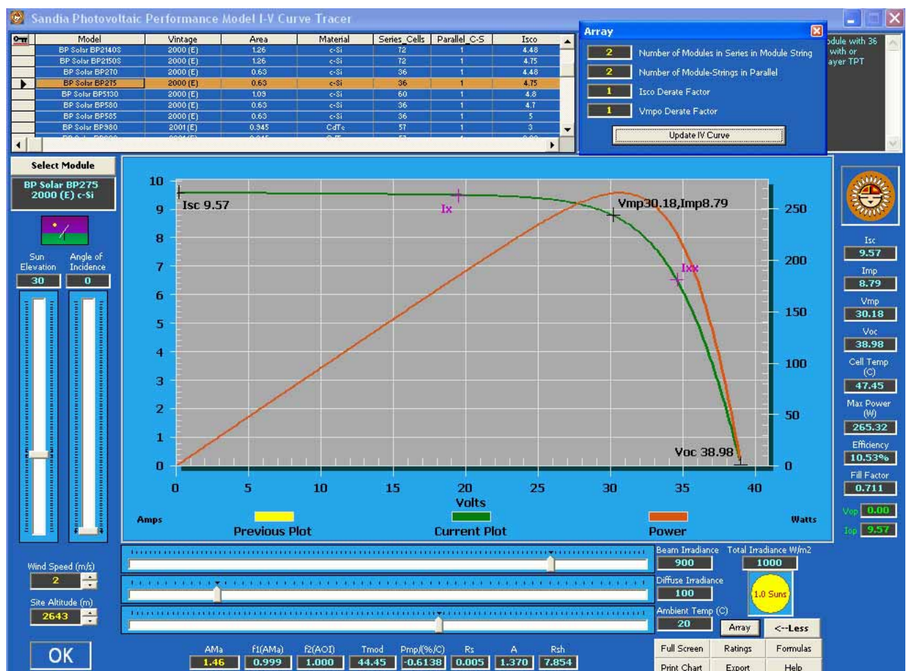
Figure 12-19: Sandia Photovoltaic Performance model I-V Curve Tracer software
