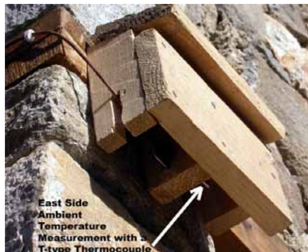
Figure 7-15: Ambient Temperature East Installed East side ambient temperature thermocouple.
