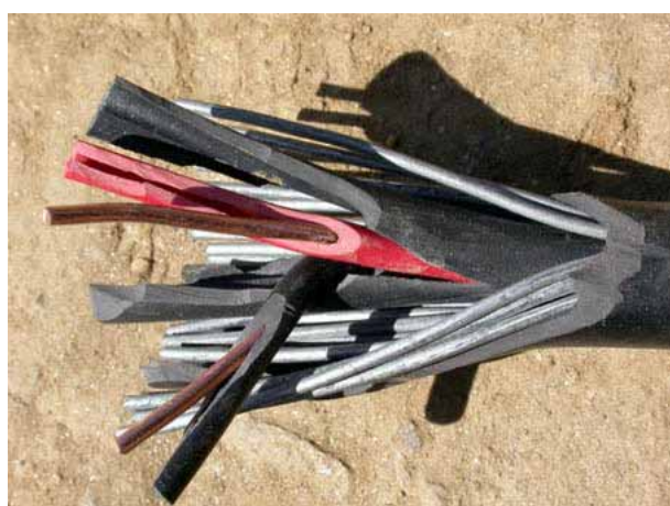
Figure 12-23: Armored cable 2.5mm 2 2.5mm 2 , 2 copper string armored cable, able to carry 32 Amp and 1,100 Volt, at up to 70° C conducting temperature.
