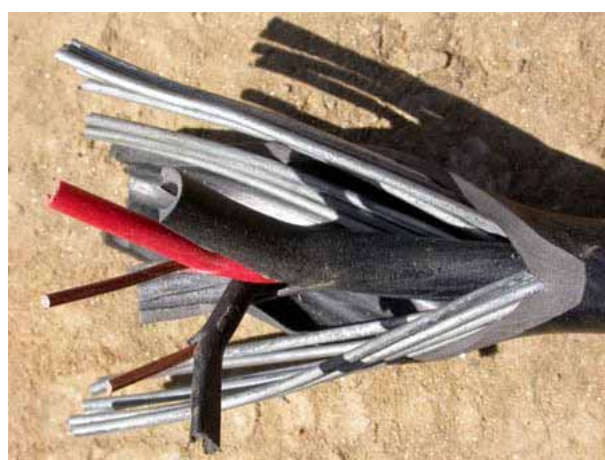
Figure 12-24: Armored cable 1.5mm 2 1.5mm 2 , 2 copper string armored cable, able to carry 23 Amp and 1,100 Volt, at up to 70° C conducting temperature.
