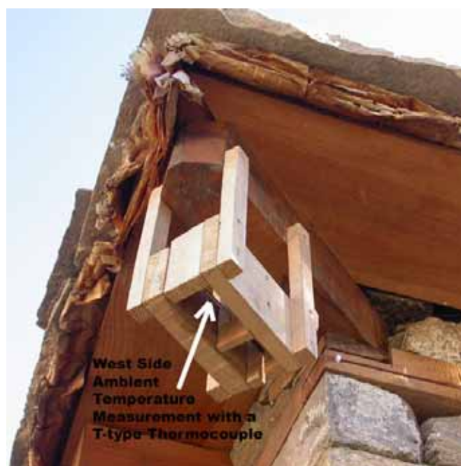
Figure 7-16: Ambient Temperature West Installed West side ambient temperature thermocouple.
