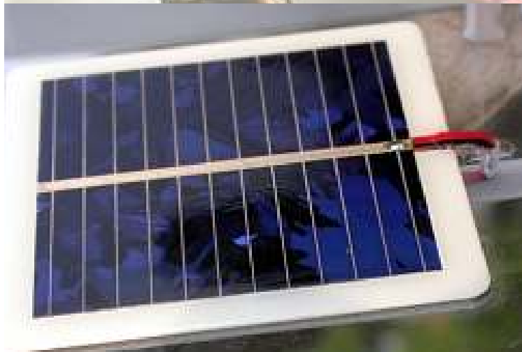
SPC 80 Pyranometer from SolData Denmark
