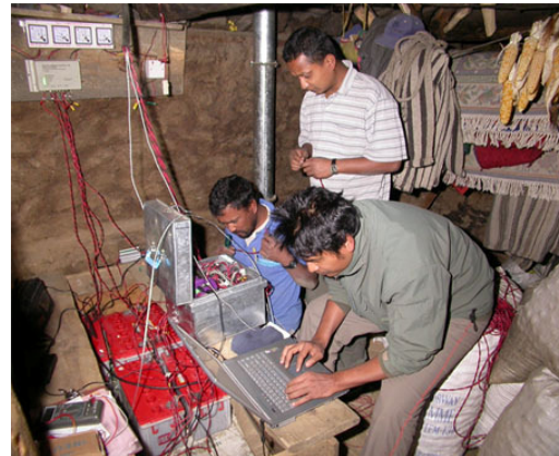
Fig. 3: Installation of the data logging system in Tulin village. The program, specifically written for the data logger DT80, is loaded and tested. The sensors' cabling is carefully connected to the data logger.
