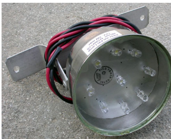
Fig. 12: 1 watt WLED (White Light Emitting Diode) lamp, manufacturing in Nepal with original Nichia NSPW 510BS diodes from Japan.
