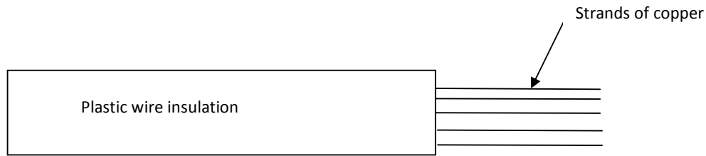
FIGURE 13: COPPER STRANDS IN PLASTIC WIRE INSULATION
