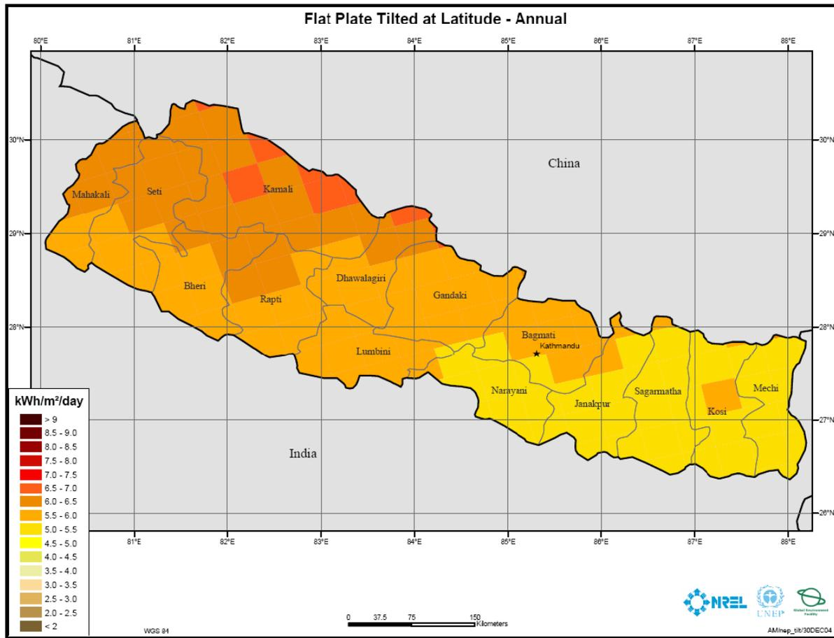
Figure 4-4: Tilted at latitude solar irradiation [kWh/m<sup>2</sup>/day] for Nepal.
