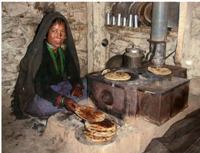
Fig 3: The Smokeless Metal Stove (SMS) which I designed in 1998, has been continually improved. Up to the end of 2010 over 5,000 homes in the remote districts of Nepal have had one installed. It cooks the traditional food “dhal bhat” all at one time and “roti”, uses ~40% less firewood, provides appropriate room heating and 9-litres of hot water for drinking the local “butter tea” as well as facilitating an improvement in personal hygiene. This is called “contextualised” technology, with people, their culture and way of living in the centre and technology developed to suit them in their context.
