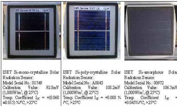
Figure 1. The three different pyranometer used to intercept the global solar radiation.
